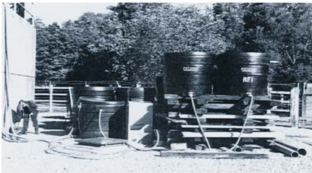
Portapak "250" enhanced slow sand filtration unit
